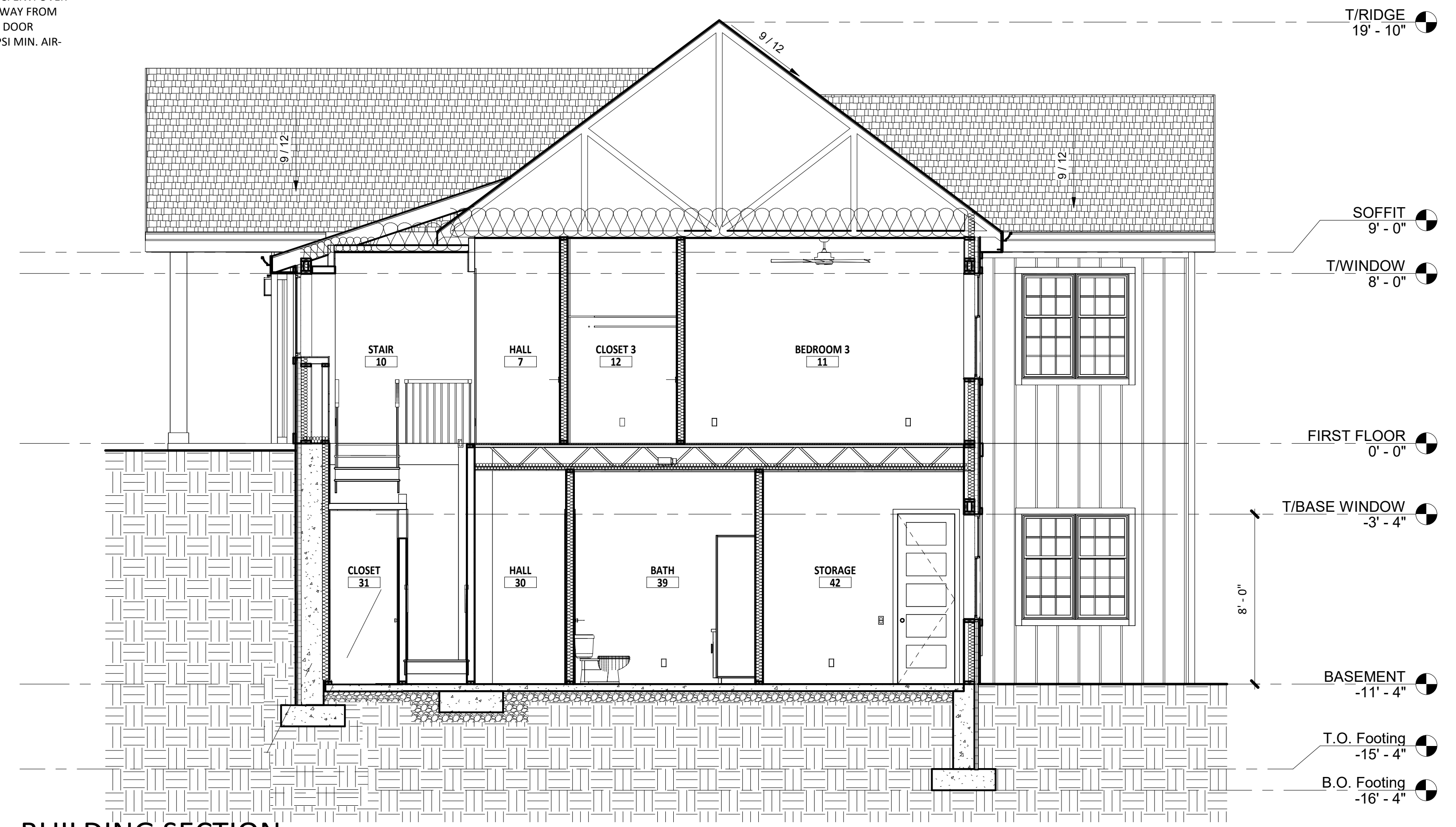
3 BUILDING SECTION SCALE: 1/4" = 1'-0"
